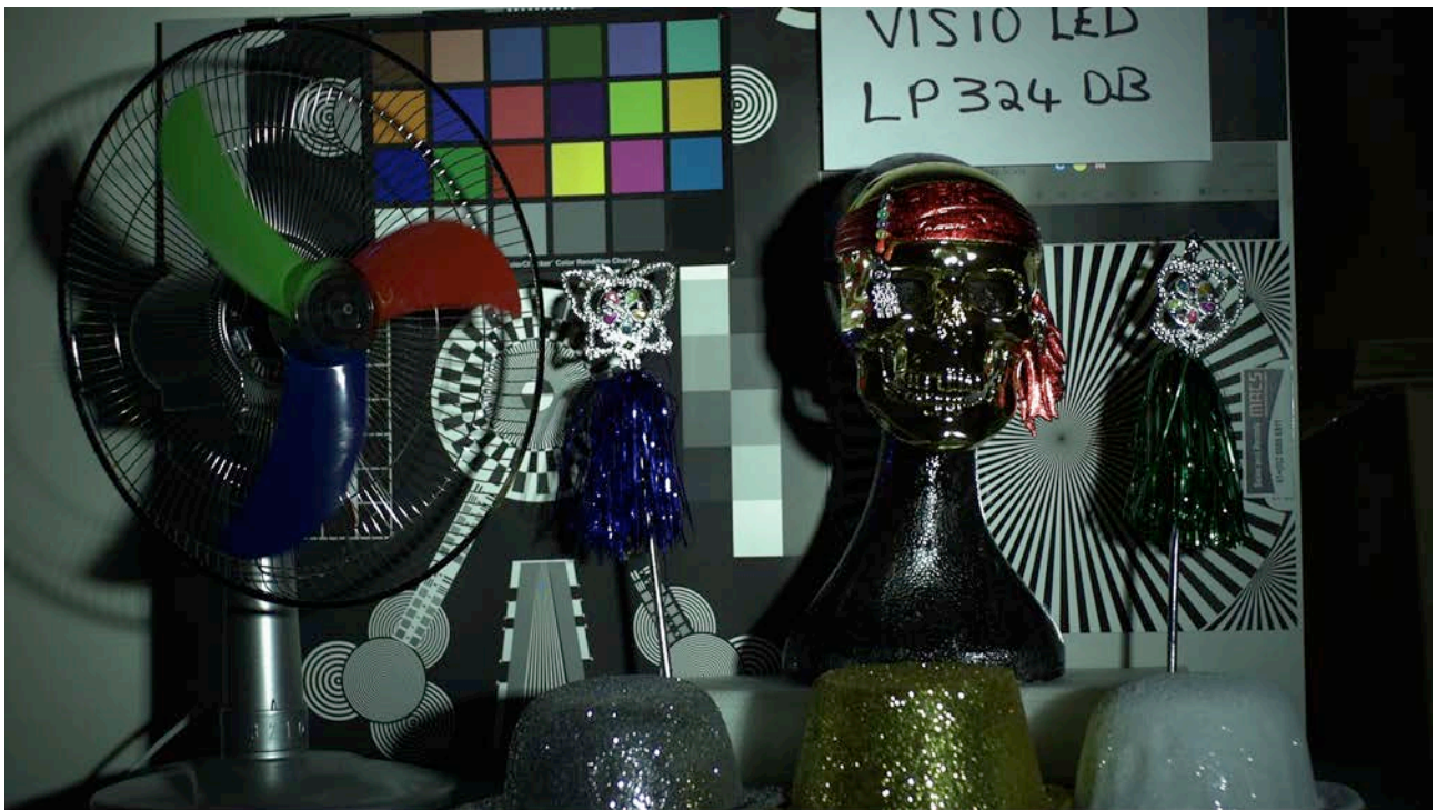
Figs. 16 and 17, VISIO 5000 LED LIGHT 10Deg. Lens, 1000fps @ f2, 6,200Deg.Kelvin with spectral response
