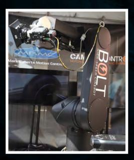
One booth that garnered a lot of attention was **Camera Control**, which presented the Bolt Cinebot for precision camera moves at ultra high speeds. The Bolt has the ability to get up to speed instantly, and go from back and forth from standstill to high-speed motion in a fraction of a second. With the Bolt arm, the camera can follow falling objects and capture images that would be impossible to do by any other method. **www.cameracontrol.com**
